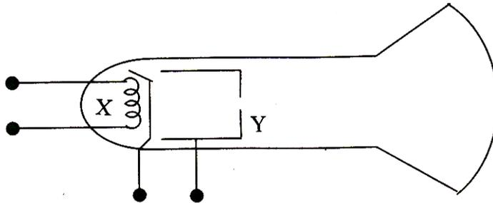
The above diagram shows an electron gun of a hot cathode ray tube,
